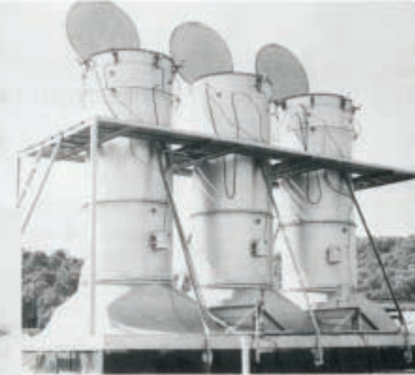
RAIN MAKING DEVICE —Rainfall up to 9" per hour can be simulated within the wind tunnel to readily determine the leakproof qualifications of various louver designs.
