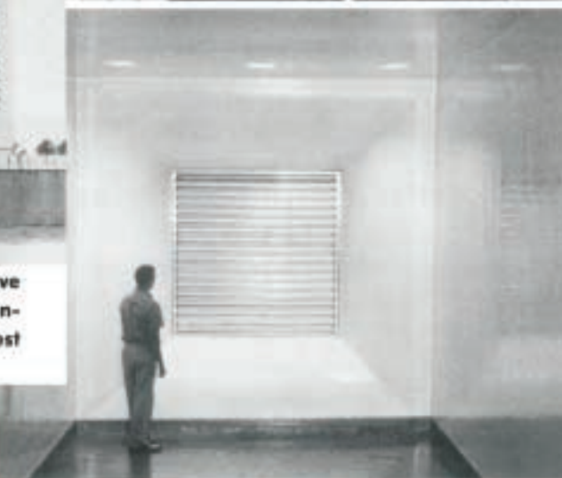
WIND TUNNEL (Interior View) —Measuring 58' from the blower to the test opening, the tunnel can test Louver sections as large as 6' wide by 6' high.
