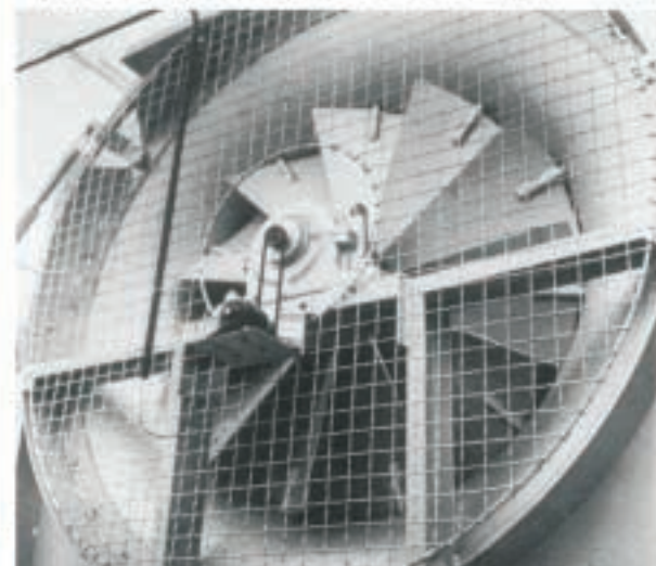
4 1/2 TON CENTRIFUGAL BLOWER —This fan, with a 66" diameter wheel and 10 position variable vanes, is capable of developing a maximum volume of 153,306 C.F.M. or a 150 M.P.H. wind.
